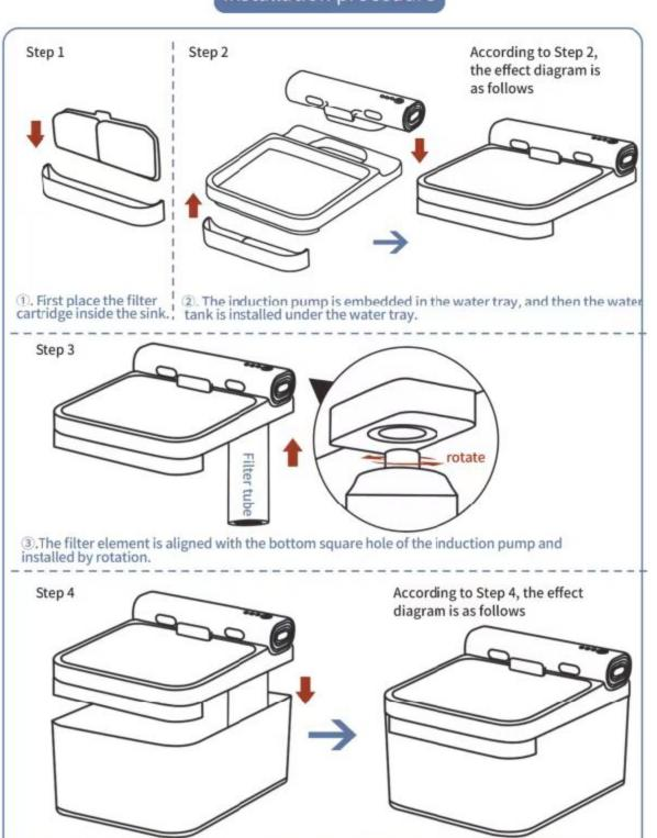
4. Finally, the induction pump and the water tray are placed above the water storage bucket
