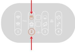
Long press for 2 seconds to start the waste bag change mode immediately.
